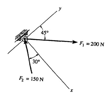
Determine the x and y components of each force acting on the gusset plate of the bridge truss. Show that the resultant force is zero.
