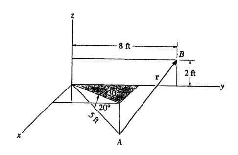
The hinged plate is supported by the cord AB. If the force in the cord is F = 340 Ib, express this force, directed from A toward B. as a Cartesian vector. What is the length of the cord?
