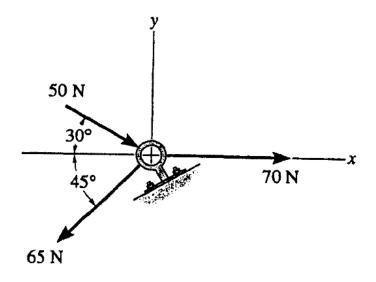
Determine the magnitude of force F so that the resultant FR of the three forces is as small as possible.
