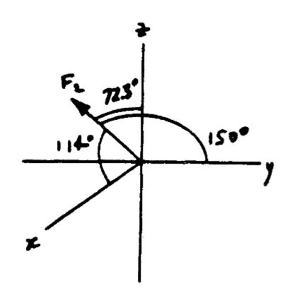
The cable at the end of the crane boom exerts a force of 250 Ib on the boom as shown. Express F as a Cartesian vector.
